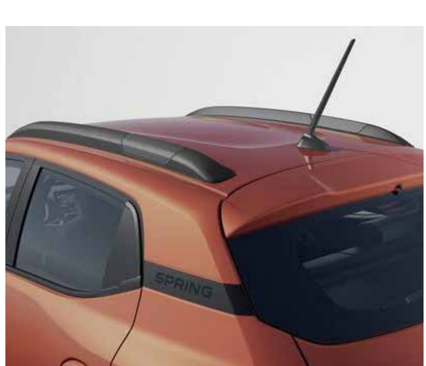
Decorative roof bars (Not load bearing)
