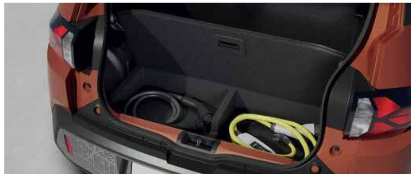
Double floor for cable storage
